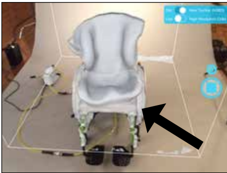
Make sure the colored foam layer of shape capture base is scanned.
